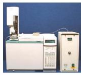
Another option is to use capillary GC-AFS for mercury speciation analysis. Absolute detection limits of 0.2 pg are easily achieved for methylmercury and ethylmercury in a variety of food samples.
